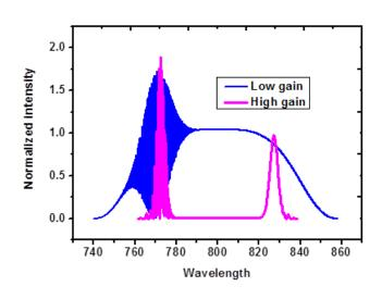
In addition we demonstrate the possibility to vary and control the spatial and spectral features of BSV and the number of modes using a nonlinear interferometer based on two nonlinear crystals separated by a certain medium. If a medium with group velocity dispersion is used it is possible "to play" with the spectral properties of the BSV light by changing both the pump power and the time delay between the pump pulse and the nonlinear signal amplified in the second crystal.
