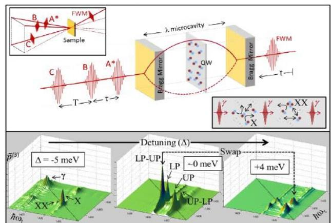
**Figure** Top panel shows the interaction with three laser pulses with the microcavity to generate a four-wave mixing signal. Bottom panel shows the resulting two-dimensional coherent spectra of the exciton (X), cavity ( $\gamma$ ) and biexciton (XX) resonances transitioning into lower- (LP) and upper-polariton (UP) modes with cavity detuning ( $\Delta$ ).
